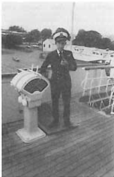
Captian Bill Warden rings up "finished with engines" on ship's telegraph after docking at Victoria.
