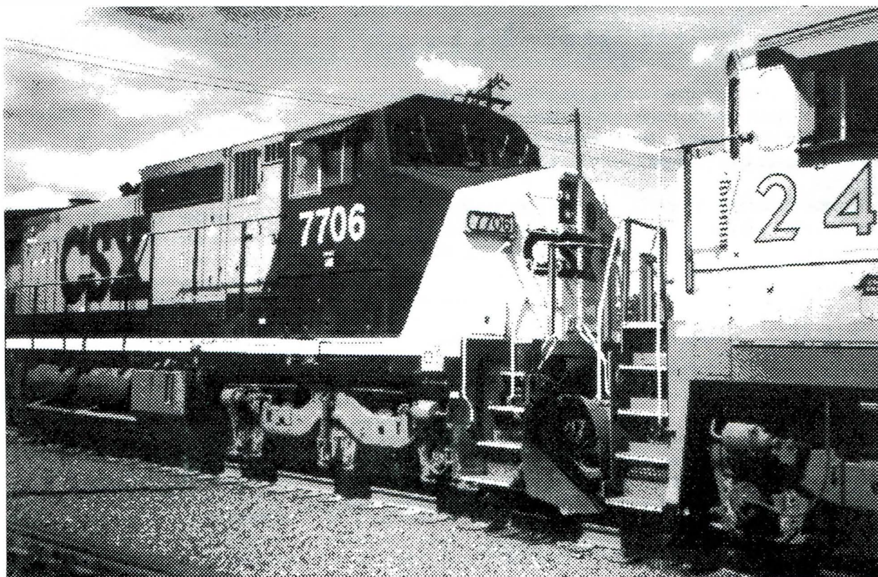
Albina Yard had many visitors during 1993. In August CSX C40-8W #7706 came to Portland amid a consist of UP power. It is shown here coupled with a 2400 series C30-7. About 17 years and 1000 HP separate these two General Electric locomotives.
