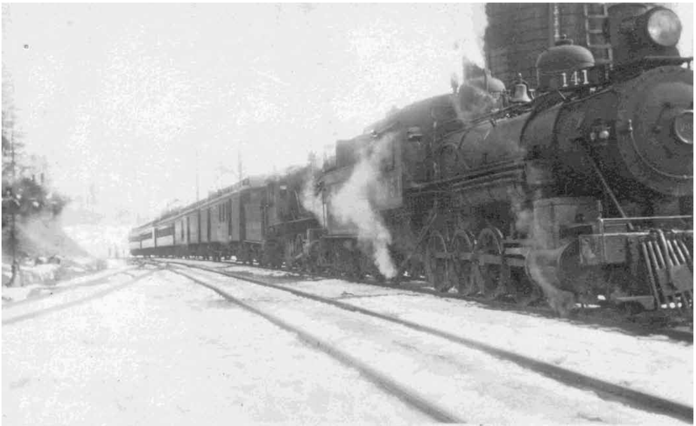
In 1921, the photographer caught train 141 at Cochran, Oregon. The 4-8-0 was built by Schenectady in 1892 and spent the last years of its operation leased to the Northwestern Pacific. The locomotive finally met the scrapper's torch in 1952. Photo, PNWC collection
