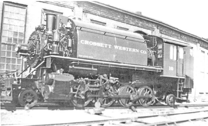
10-3J ALCO 2-8-2T Crossett-Western Co. CN-67652 at Livingston, MT enroute to Wauna, OR MAR 1929 DSR 3-1 (Courtesy of PNWC Archives)
